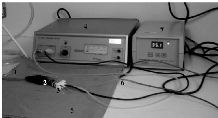
**Figure 2.2** Anesthetic setup. 1- oxygen delivery tube; 2- mice in dorsal recumbence, 3- cuff and transducer; 4- pulse rate and blood pressure meter, 5- drape covering the homeothermic blanket; 6- rectal probe to measure temperature; 7- device to measure the temperature. Figure original of the author.
