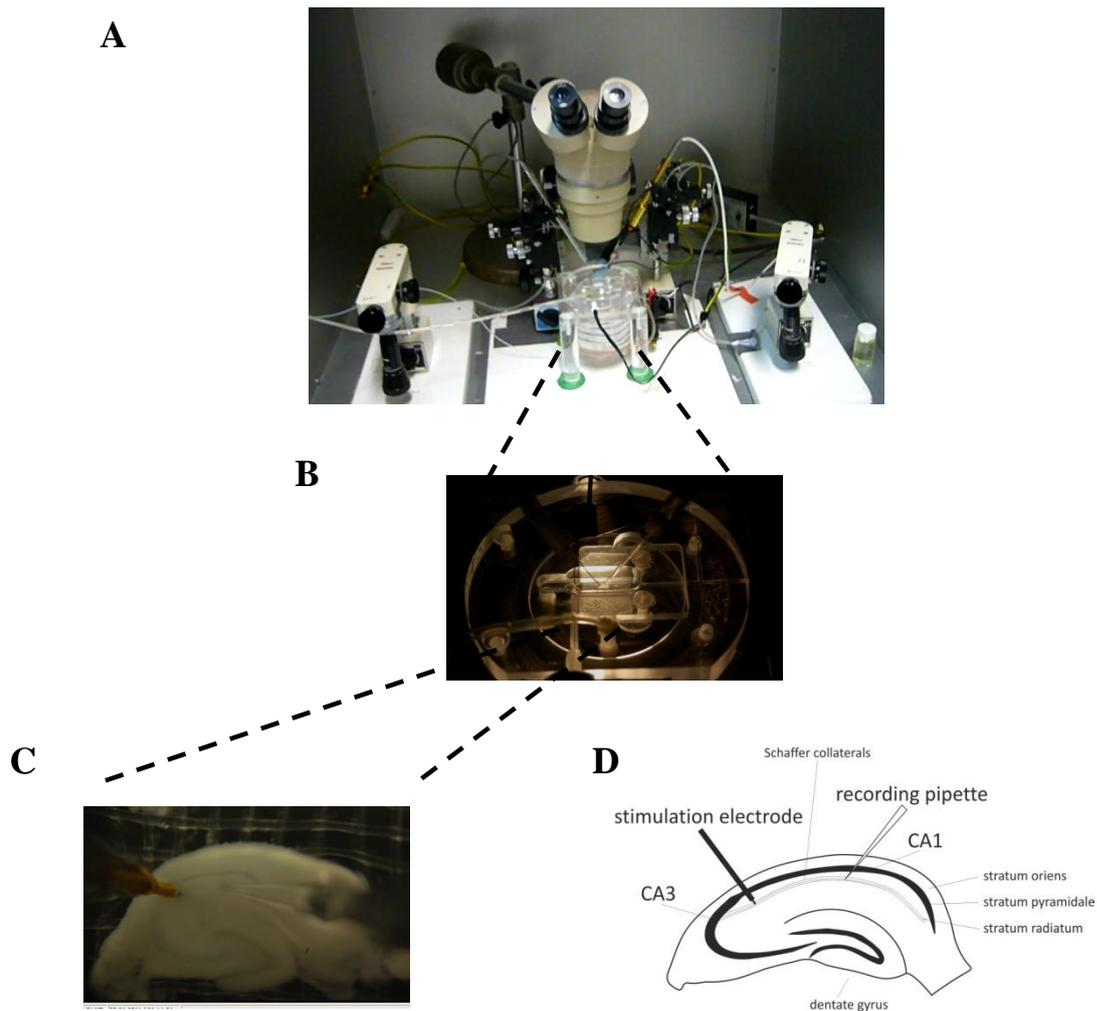
**Figure 2.8** A- Electrophysiological setup, B- Acrylic camera with a hippocampal slice, C- Hippocampal slice, stimulating electrode and recording pipette. The recording pipette was placed in the stratum radiatum of the CA1, and the stimulating electrode was placed in the stratum radiatum near the CA3/CA1 border to stimulate the Schaffer collateral pathway. D- Schematic figure of a hippocampal mouse slice with the stimulating electrode and recording pipette. Figure original of the author.
