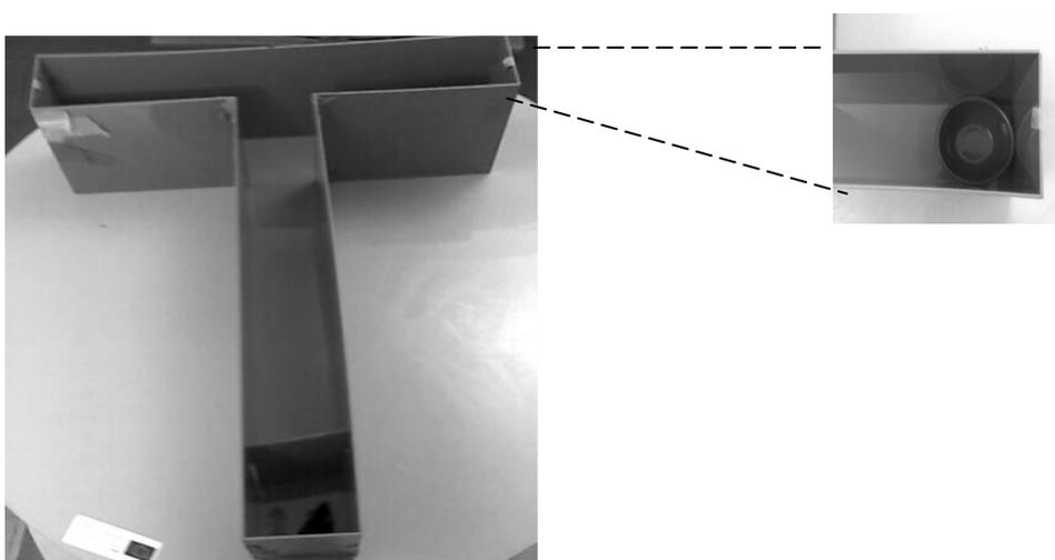
**Figure 2.5** T-maze apparatus. Figure at the right represents the magnification of the right arm of the T-maze with the ceramic food pot. Figure original of the author.
