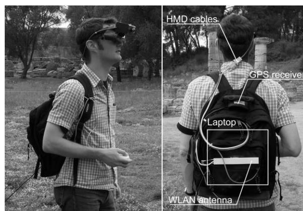
Figura 12 MARS do projeto ARCHEOGUIDE, vista frontal e traseira (Gleue & Dähne, 2001)
