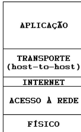
**Figura 2.2** – Modelo TCP/IP
