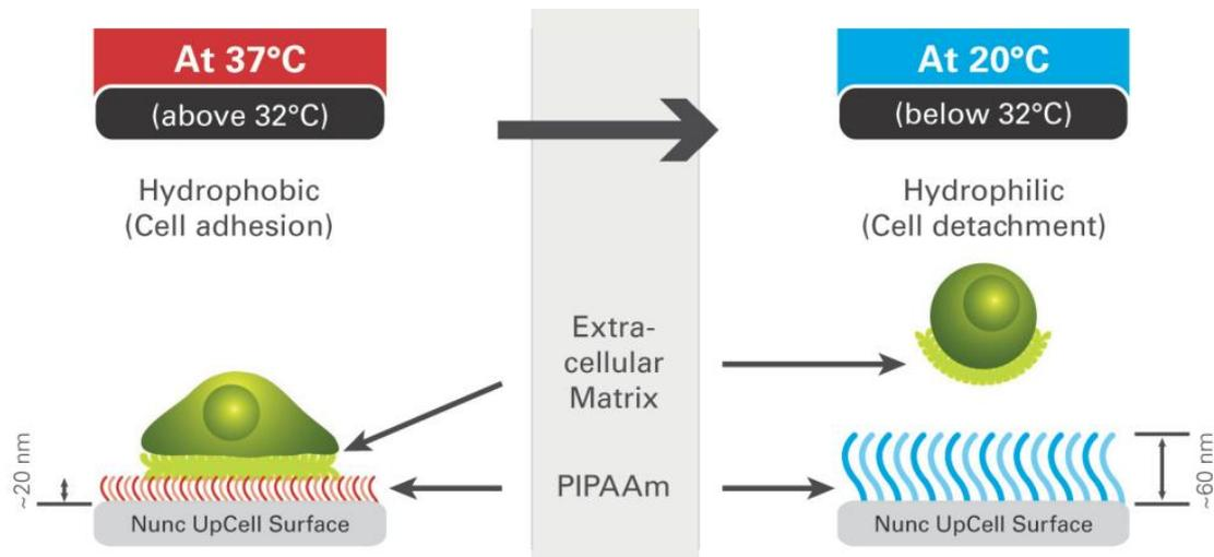
**Figure 1** – Features and functioning of TR surfaces. Adapted from Thermo Scientific Nunc UpCell Surface manual.
