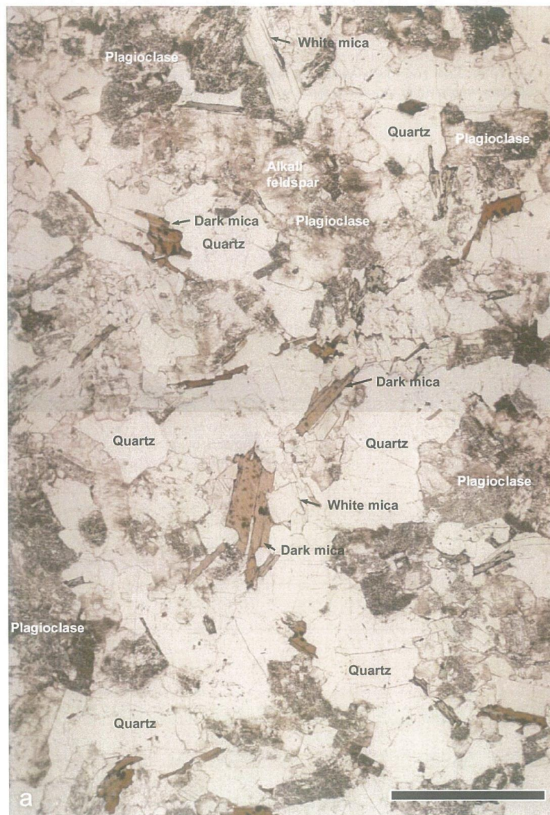
Figure 2a: Polarizing microscopical overview photo micrograph. Major part of the rock consisting of alkali feldspar, plagioclase, dark mica (biotite) and white mica (muscovite), partially intergrown in aggregates, xenomorphic quartz in aggregates. Relatively finer grain size of plagioclase in interstitials between quartz. Plane polarised light. Scale bar corresponds to 2 mm length. Field width 7.2 mm. Thin section LGA136-182.
